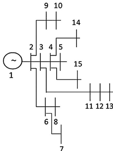
**Figure 1: One line diagram of IEEE 15-bus RDS.**
