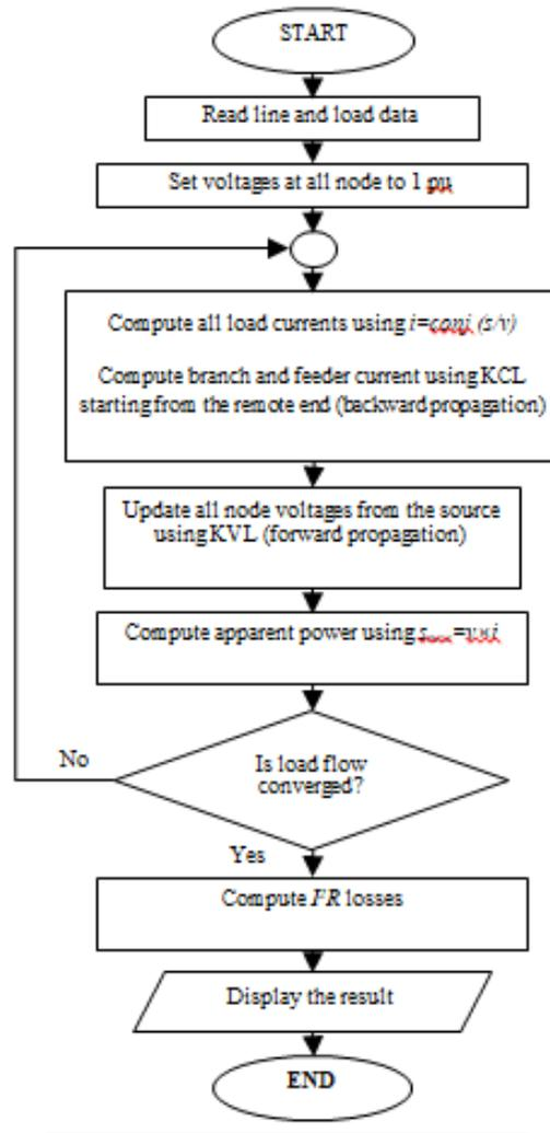
**Figure 3: Flowchart of backward-forward sweep load flow algorithm.**
