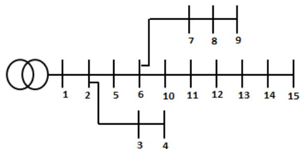
**Figure 2: One line diagram of the Nigerian 11 kV network.**
