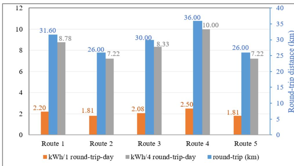
**Figure 3: Comparison of energy demand for one and four round-trips at different routes.**
