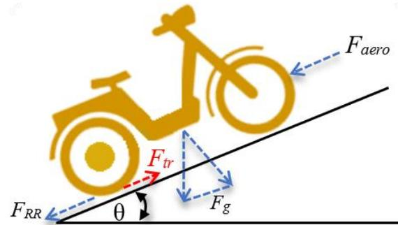
Figure 2: Resisting forces acting on an e-motorcycle.
